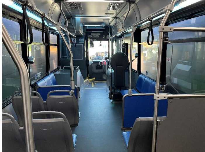
Figure 5.6: Overview of ADA securement area in the front of the Flash vehicle, showing two securement positions with flip-up bench seating and the rear-facing Q'straint Quantum automatic securement position (right side of image).
