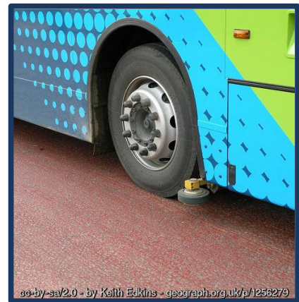
Figure 4.19: Cambridge Guided Busway Sensor Wheel (source: © Keith Edkins)
