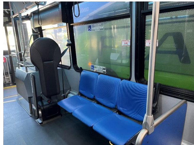
Figure 5.7: Automated rear-facing ADA securement position with flip-up bench seating
