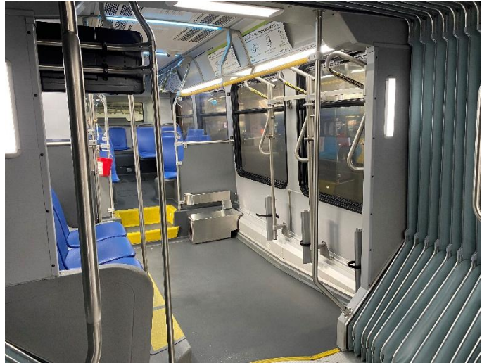
Figure 5.9: View of the roll-aboard bicycle stowage area opposite the rear door.
