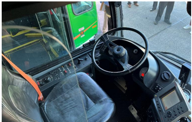
Figure 5.8: Operator Compartment, with portion of the protective partition visible in the foreground.
