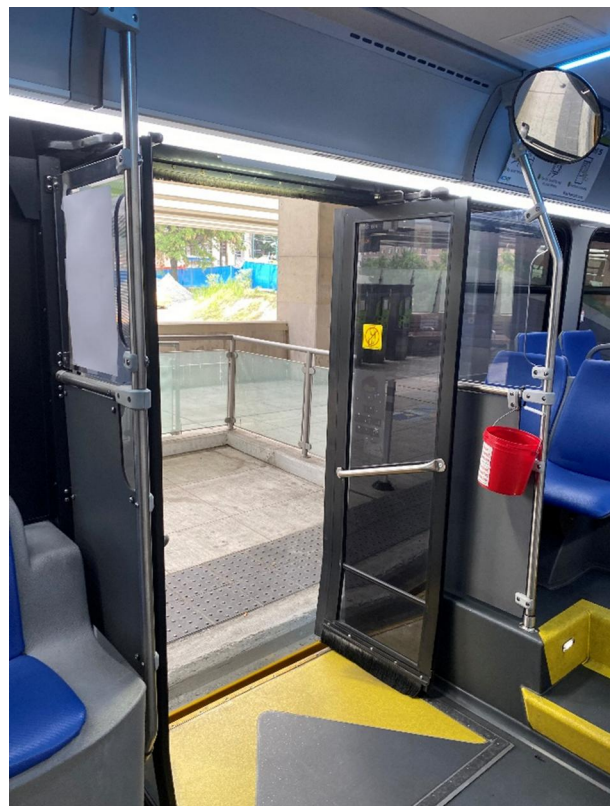
Figure 5.4: Rear door position showing near-level boarding with the station platform, deployable bridge plate, and wide doors to reduce doorway obstruction
